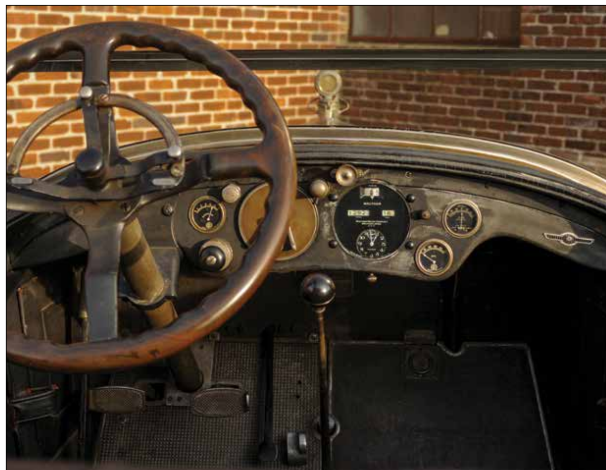
Just like today, some of the controls are on the steering wheel. New instrumentation for the 3-25 model which carried over to 3-35: Ammeter, oil and gas pressure gauges, speedometer and clock. Manual 3-speed tranny, Semi floating differential; spiral bevel gears; rear axle ratio 4.36. Power steering, power brakes and automatic shift trans were still a few years away. This was the era of the pro chauffeur.
